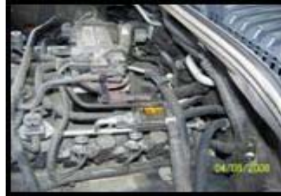
Unit installed on Hose just before Silver 1ft long Injector Fuel Rail (Left); Right-Unit installed on Black Flex Hose before Fuel Inj.
