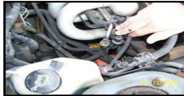
Unit Installed on a small car 1999 year Mazda Designed Engine. Installer has fingers on silver fuel line On Engine Topside, Cause that's where fuel rail on this engine comes up from underneath. Also seen is the FuelMaster SD installed on the fuel hose flex section just before the fuel rail goes to the Engine. Easy to install & most small car fuel lines are similar set ups for 4cyl.
