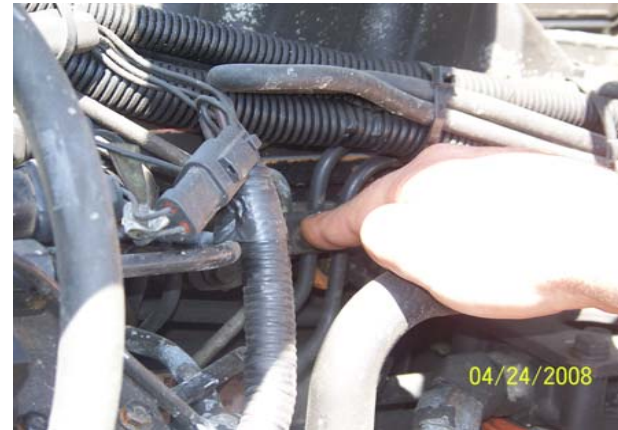
On Big Rigs or Top Kicks: Install 3 XL's On Fuel Line Where Installers Fingers are left or Right one per Injector line.
